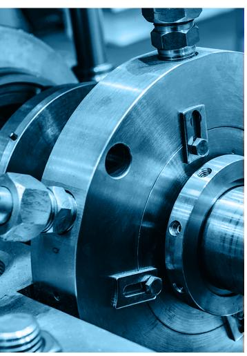
A mechanically loaded device consisting of rotating and stationary members, having lapped faces operating in close proximity under hydraulic load, used to minimize leakage between rotating shaft and stationary housing.
